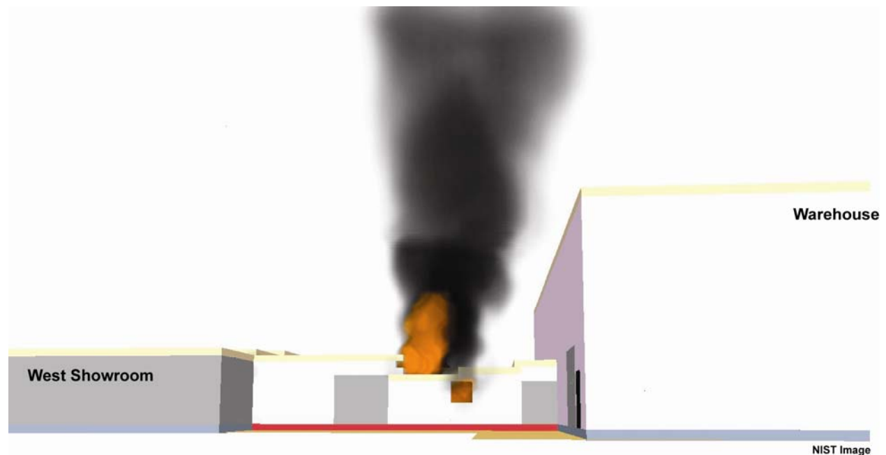
Figure 4-11. Rendered image showing the west side of the loading dock 110 s into the simulation.
