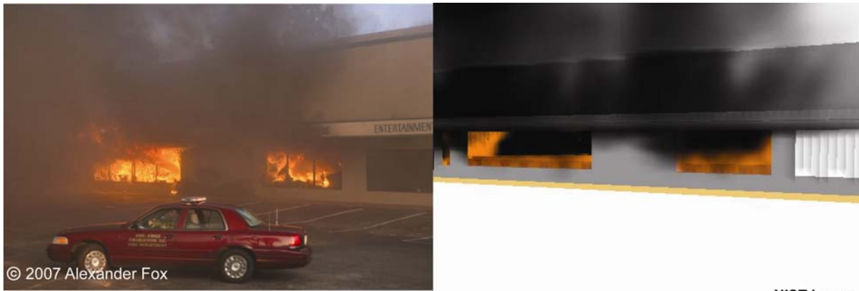
Figure 4-23. Comparison between photo and rendered image from the simulation at 1686 s (7:38:59 p.m.). The view is of the front of the main and west showrooms.
