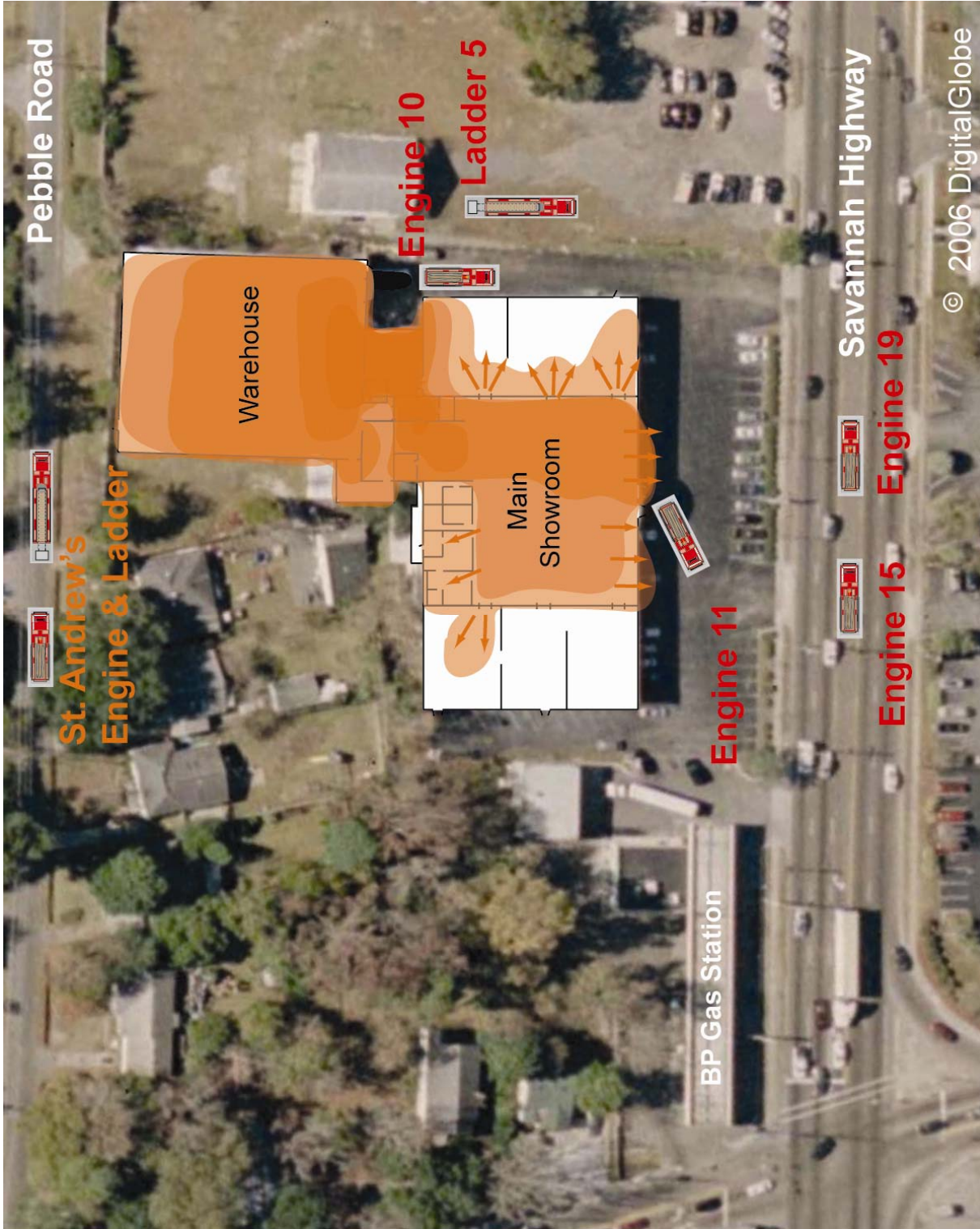
Figure 2-10. Fire spreading to west showroom and the rear of east showroom. This occurred by about 7:38 p.m. Background image used with permission of DigitalGlobe. Enhancements by NIST.
