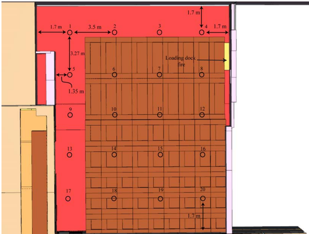
Figure 4-35. Sprinkler layout inside the enclosed loading dock.
