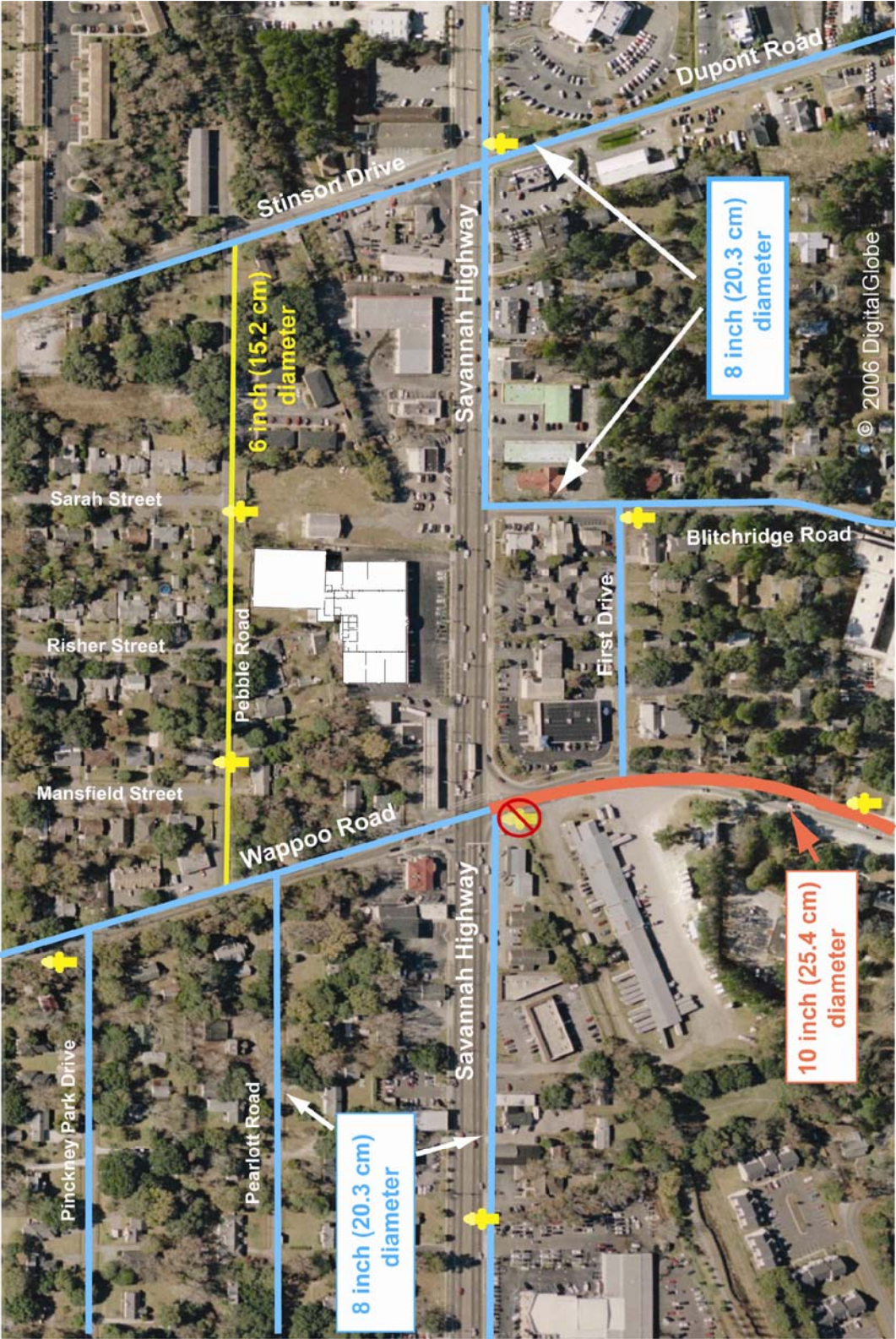
Figure 1-18. Water supply lines near Sofa Super Store. Hydrants behind store on Pebble Road were on 15.2 cm (6 in) diameter lines while hydrants located along Savannah Highway were on 20.3 cm (8 in) diameter lines. Background image used with permission of DigitalGlobe. Enhancements by NIST.
