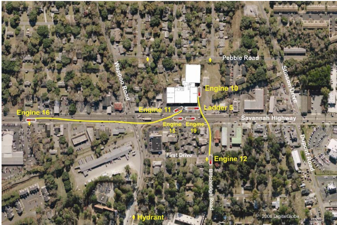
Figure 2-2. Positioned at fire hydrants on Savannah Highway and Blichridge Road, Engines 16 and 12 were pumping water to Engines 10 and 11 at about 7:27 pm. Background image used with permission of DigitalGlobe. Enhancements by NIST.
