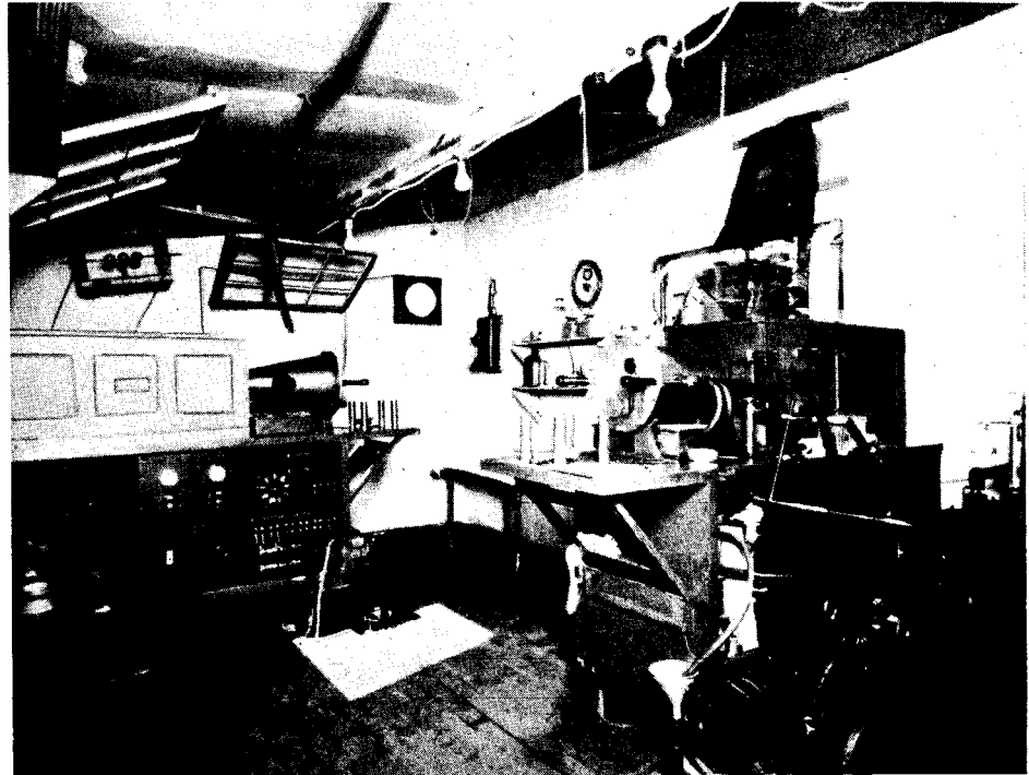
Fig. 17. The Two Cathode-ray Oscillographs in the Lightning Laboratory of 1929. (See Fig. 14)
