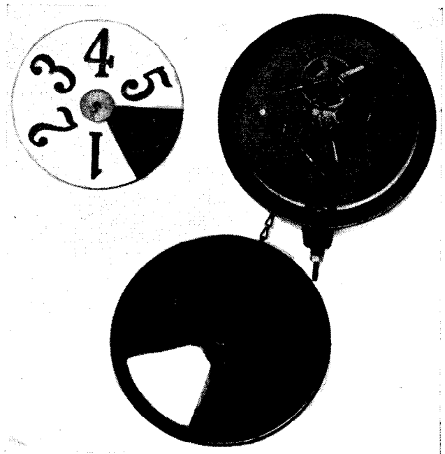
Fig. 32. Interior of the Surge Indicator Shown in Fig. 31
