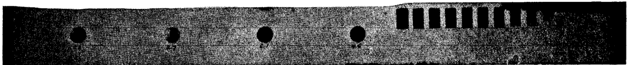
Fig. 35. Type of Record Made by the Lightning-severity Meter
