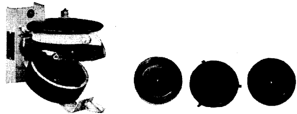
Fig. 10. Stationary-film Type of Surge-voltage Recorder with the Porcelain Housing and Film Container Open
