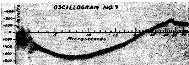
Fig. 23(d). Cathode-ray Oscillogram Taken on July 19, 1929. This is a wave which has a slightly oscillatory nature and is typical of a large group of waves. A cloud-to-ground stroke was seen at the instant this oscillogram was obtained. This stroke was at least 10 miles distant from the laboratory and some distance from the line
