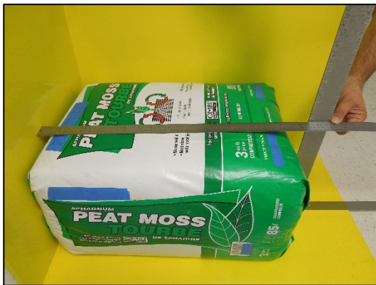
Figure 3-5. Height Measurement. The packaging tail on the end of the package can affect this measurement so it has been folded over and taped against the end of the package.
