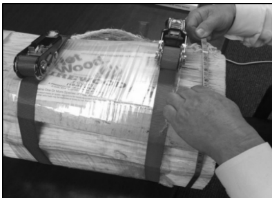
Figure 3-13a. Strapping the Ends of a Bundle.
