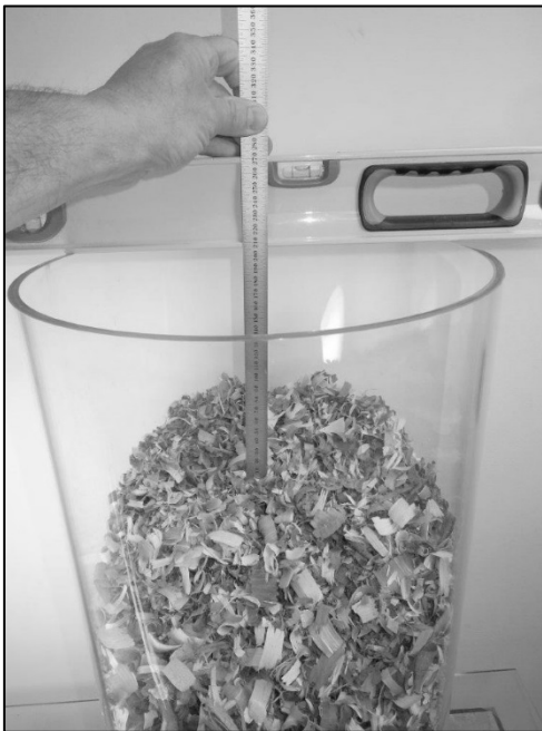
Figure 3-26. Placing the Ruler into the Test Measure with Zero End Down.
