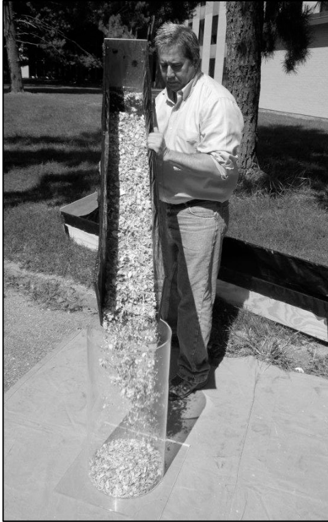
Figure 3-23. Filling a 44 L Test Measure.
