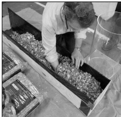
Figure 3-20. First Pour into the Test Measure.
