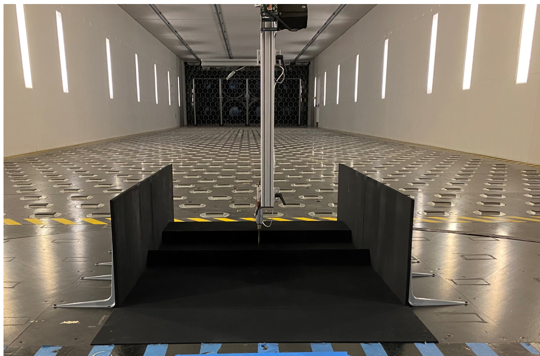
Wind Tunnel Testing of Generic Terraced Model
