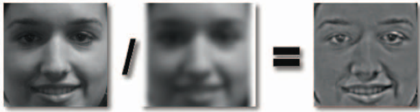
Fig. 7. This figure illustrates the computation of a self-quotient face image. The face image to the left is a cropped and geometrically normalized image. The image in the middle is the geometrically normalized image blurred by a Gaussian kernel. The image on the right is a self-quotient image. This image is obtained by pixel-wise division of the normalized image by the blurred image.
