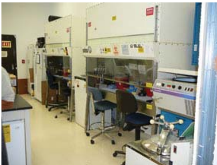
Bio-safety Cabinets for BNA extractions are Class II Type A HEPA filtered recirculated room air cabinets. Class II B3 HEPA filtered exhausted to outdoor cabinets are preferred.
