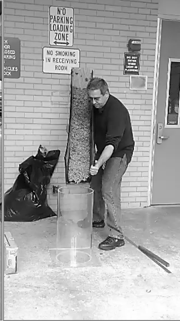
Exhibit 25. Photo to the left shows the use of a chute to pour shredded paper bedding into a 44 L (1.5 cu ft) test measure.
