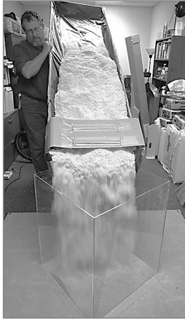
Exhibit 24. Photo to the right shows the use of a chute to pour small flake bedding into a 283 L (10 cu ft) test measure.
