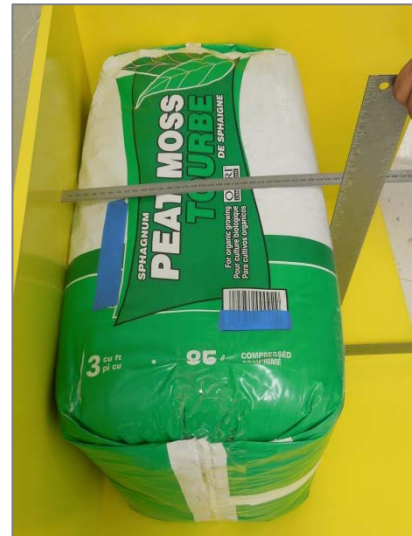
Exhibit 9. Width Measurement – the frame is rotated on its end to vertical so that the carpenter square does not compress the product.
