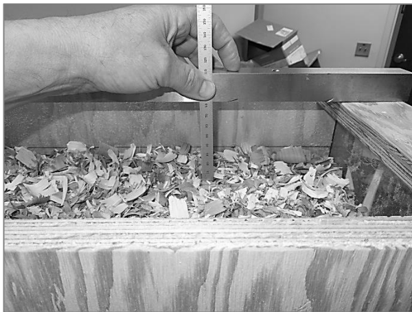
Figure 3. Using the headspace measurement on 56.6 L (2 cu ft) test measure. The ruler is read from the bottom edge of a straight edge or level from a position that reduces parallax.
