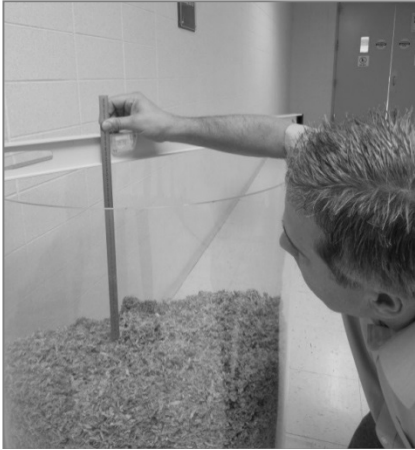
Figure 3. Using the headspace measurement on a 279 L test measure. The ruler is read from the bottom edge of a straight edge or level from a position that reduces parallax.
