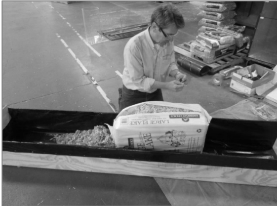
Exhibit 26. These pictures show a package of bedding being opened and the product being uncompressed and prepared for measuring.
