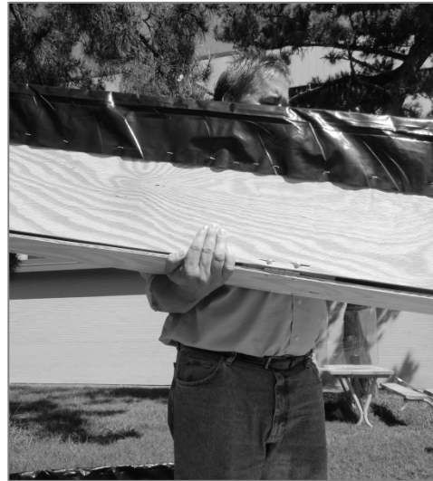
Exhibit 14. Showing how to cradle the chute on one arm and holding it with one hand while tilting it with the other hand.
