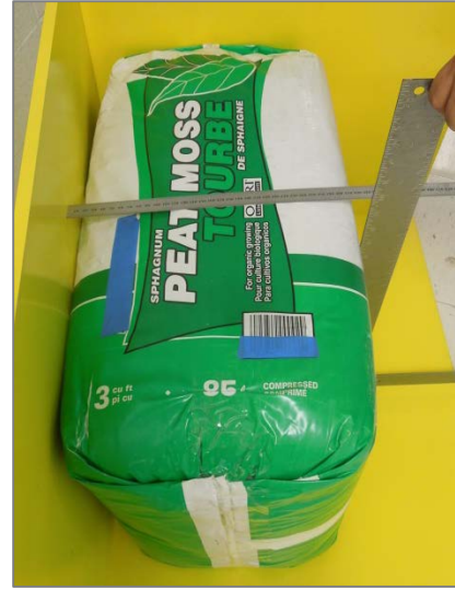
Figure 3-6. Width Measurement – the frame is rotated on its end to vertical so that the carpenter square does not compress the product.
