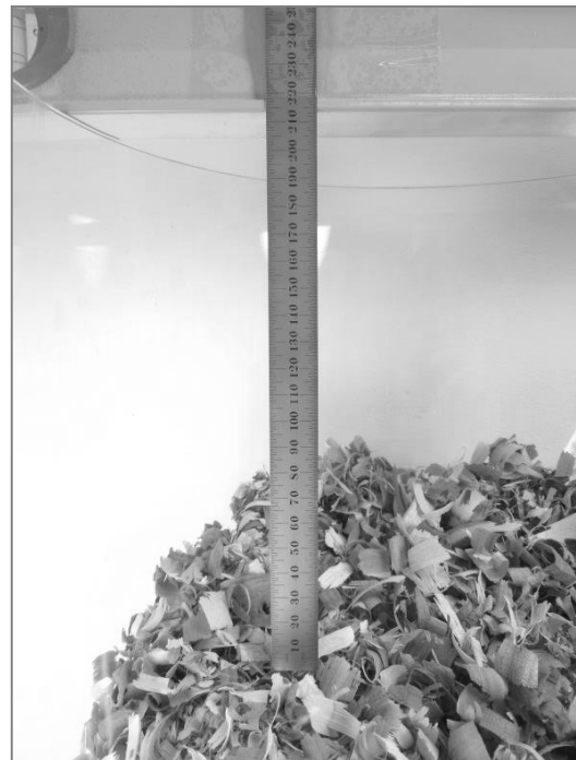
Exhibit 19. Ruler shown with zero end at surface of the bedding.
