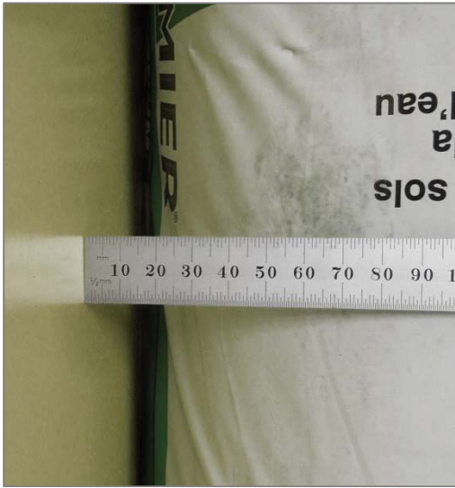
Exhibit 6. The rigid frame allows the observer to hold the zero reference point firmly in place.
