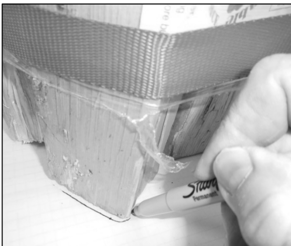
Figure 8. Tracing the Perimeter of the Wood.
