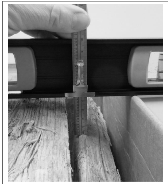
Figure 2.a. – Examples of the Headspace Measurement
