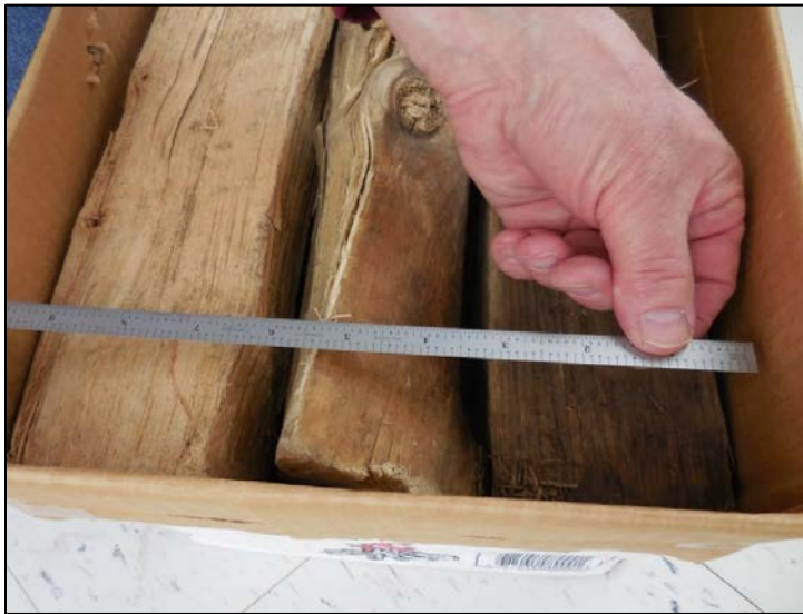
Figure 3b. Measuring the Width of the Firewood in a Box.
