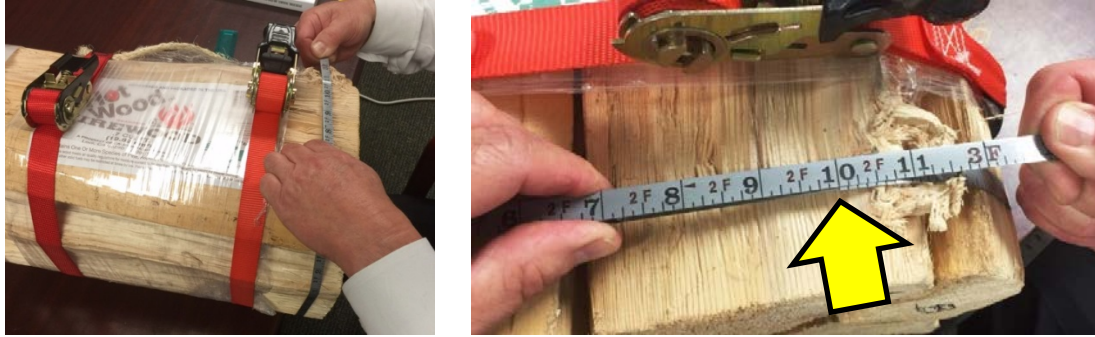
Figure 15. Strapping the End of a Bundle.
