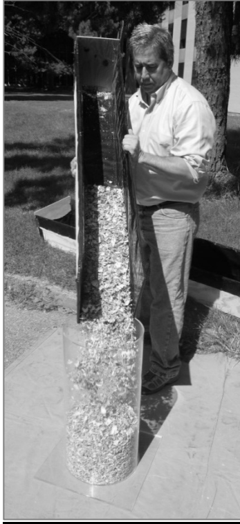
Exhibit 6. Filling a 44 L Test Measure.
