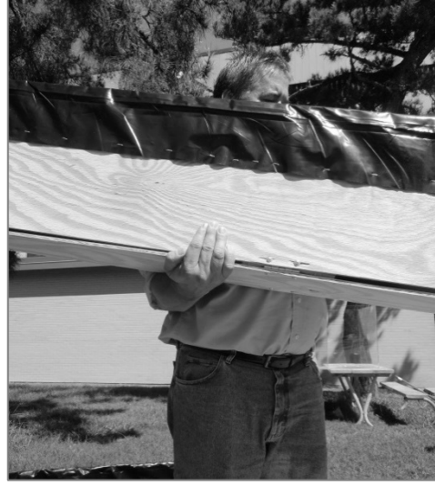
Exhibit 5. Showing how to cradle the chute on one arm and holding it with one hand while tilting it with the other hand.
