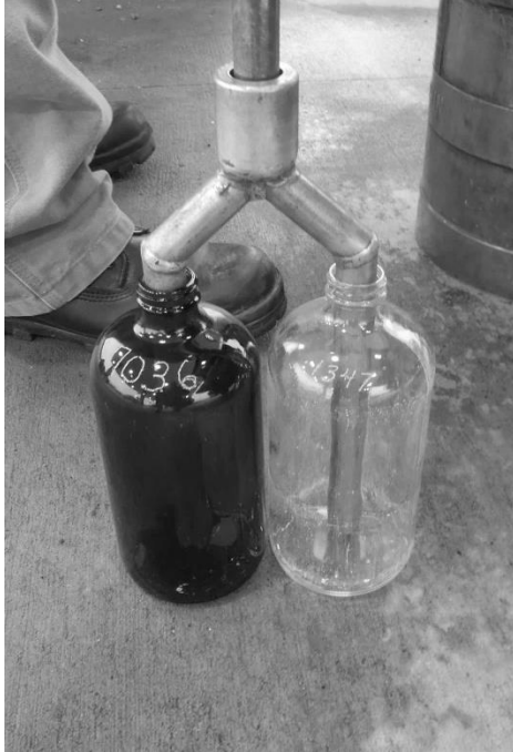
Figure 19. Sample Bottles Empty and Filled with Bifurcated Tube.
