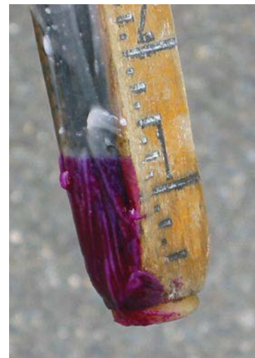
Figure 26. Sticks with Red Coloring that Shows Water Levels in Different Storage Tanks.
