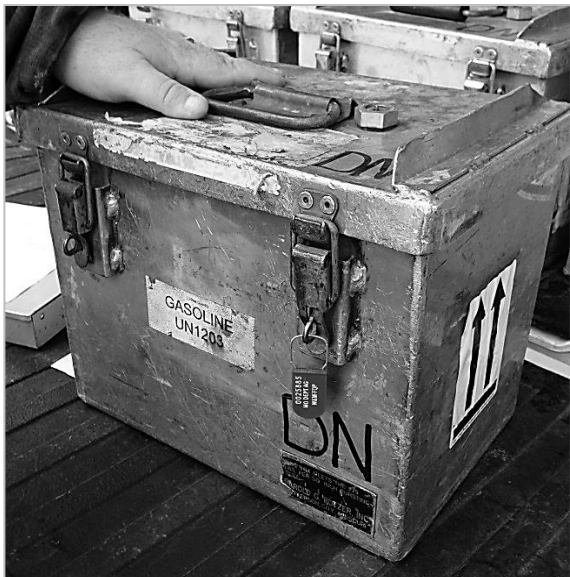
Figure 13c. Sample Box showing Security Seal in Place
