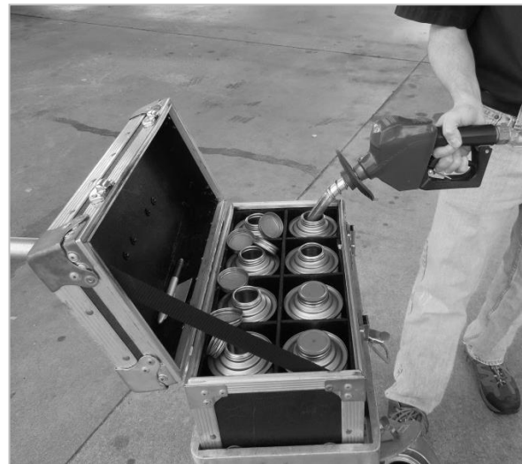
21. Fuel Sampling Cart with Sample Container bonded to cart and ground.*
