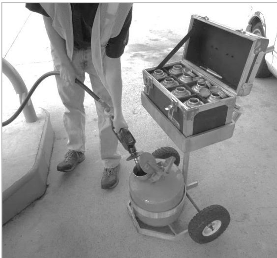
20. Fuel Sampling Cart with Transport Case and Safety Gasoline Can to hold fuel from nozzle-hose flushes.*
