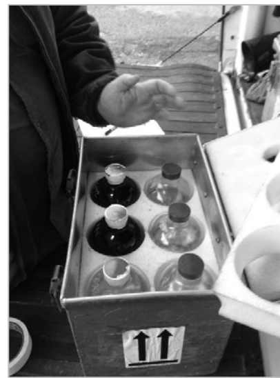
Figure 16b. Sample Box Showing Insulation.
