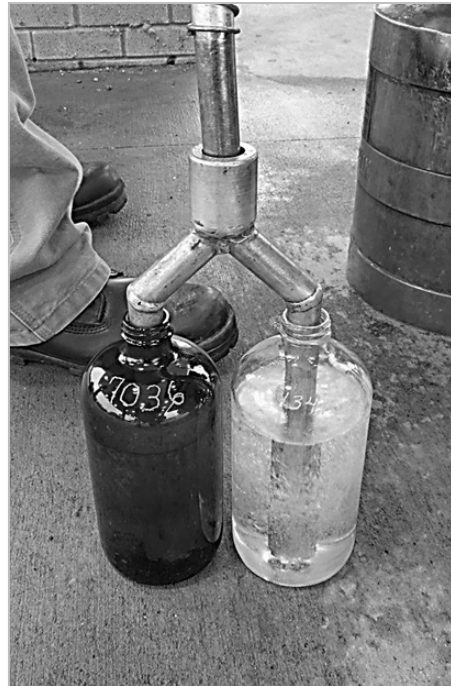
Figure 19. Sample Bottles Empty and Filled with Bifurcated Tube.
