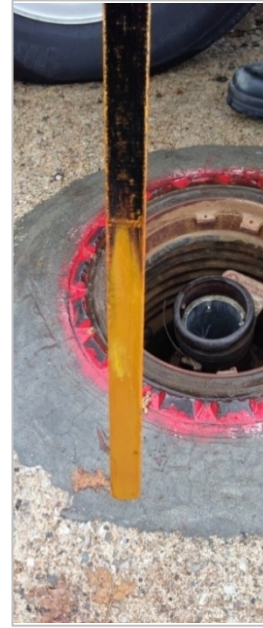
Figure 25. Stick with Paste – No Water Indicated.
