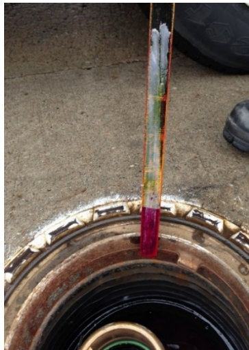
Figure 26. Sticks with Red Coloring that Shows Water Levels in Different Storage Tanks.
