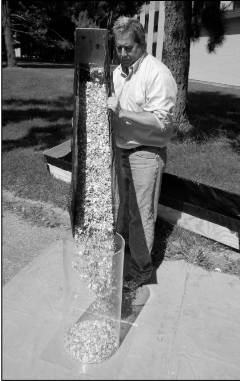
Figure 3-23. Filling a 44 L Test Measure.
