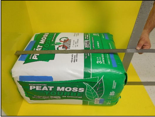
Figure 3-5. Height Measurement. The packaging tail on the end of the package can affect this measurement so it has been folded over and taped against the end of the package.
