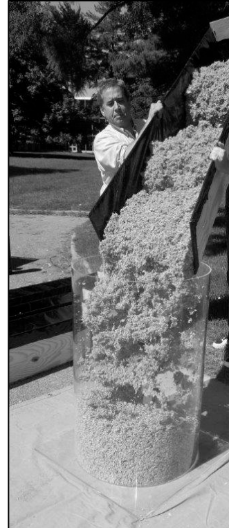
Figure 3-24. Filling a Test Measure at an Angle to use the Larger Opening.
