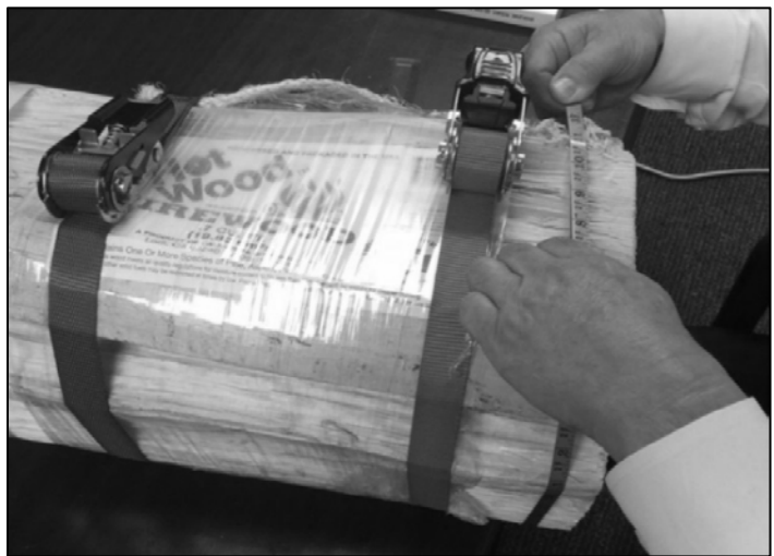
Figure 3-13a. Strapping the Ends of a Bundle.
