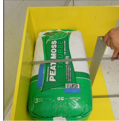
Figure 3-6. Width Measurement. The frame is rotated on its end to vertical so that the carpenter square does not compress the product.
