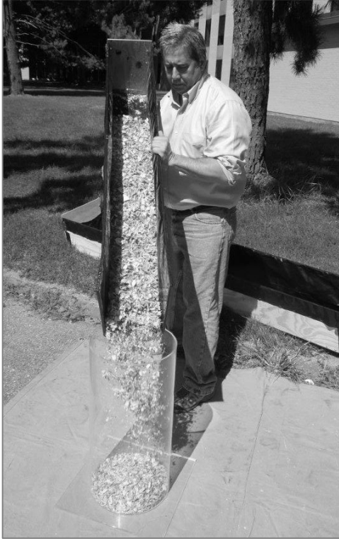
Figure 3-23. Filling a 44 L Test Measure.
