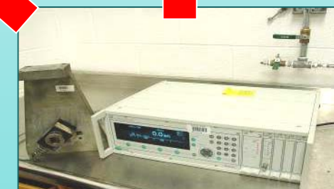
Transfer Lab MGC Plus Torque Readout & Cell Uncertainty: 0.5 %
