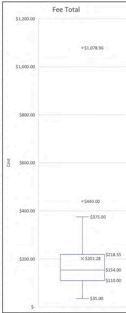
Figure 29: Fees charged for testing a 31 lb weight kit containing 22 pieces to NIST HB 105-1 Class F tolerances using mass echelon III procedures.
