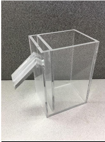
Figure 3-7(a). Example of a Displacement Vessel.
