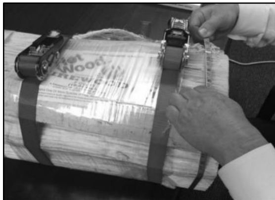
Figure 3-13a. Strapping the Ends of a Bundle.
