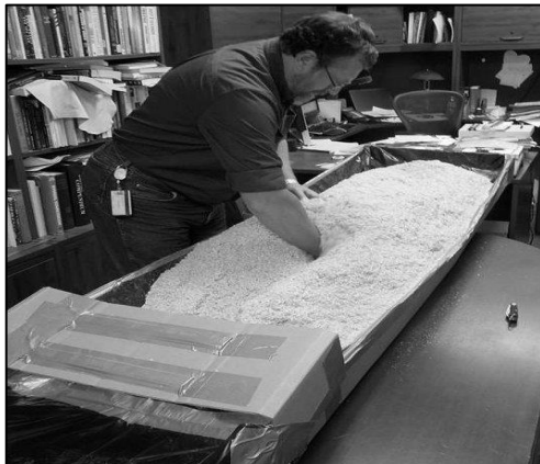
Figure 3-18. Spreading Bedding Material
