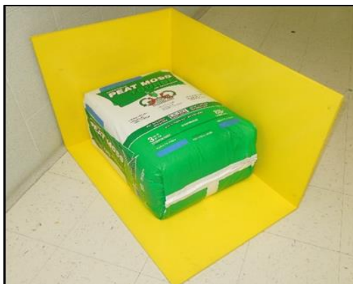
Figure 3-1. Dimensional Measuring Frame
