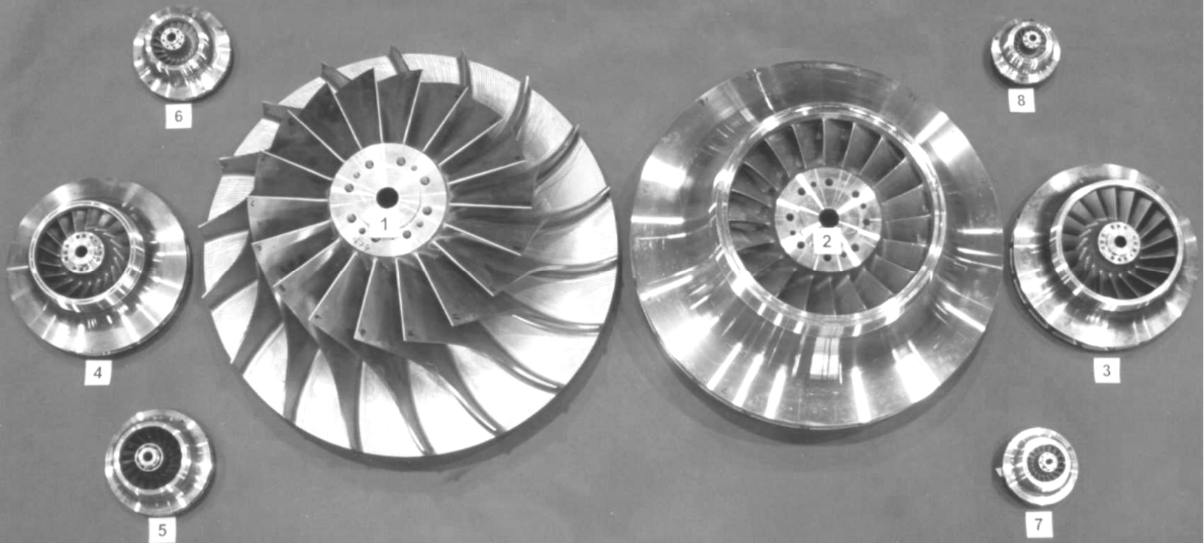
Integrally Geared Centrifugal Impellers: Stages 1 through 8
