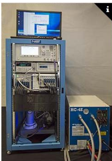
Cryocooled NIST Programmable Josephson Voltage Standard system for realizing intrinsically accurate DC voltages from -10V to +10V. Available as a NIST Standard Reference Instrument .
