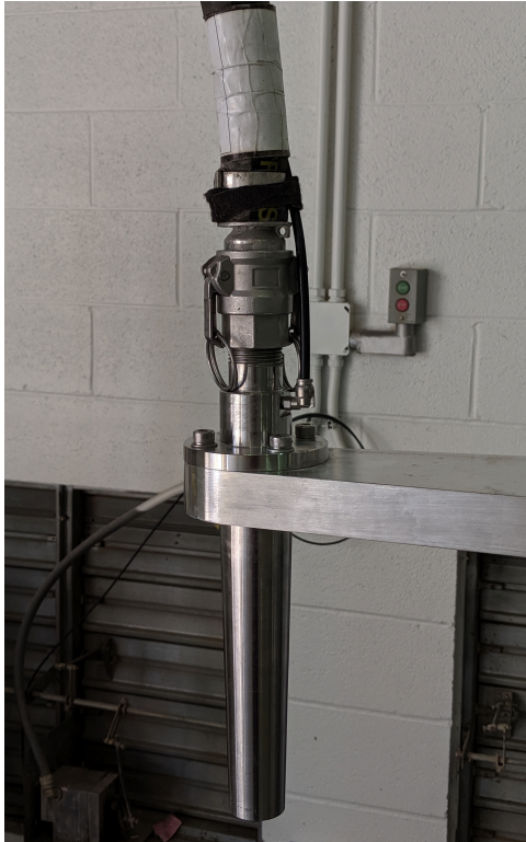
Left: The single component nozzle with 23 mm ID. Right: Two-component mixing nozzle. Component 1 is supplied by the grout pump and component 2 is supplied by user-supplied hardware.
