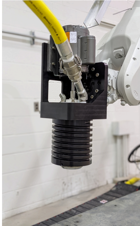
Left: The single component nozzle with 23 mm ID. Right: Two-component mixing nozzle. Component 1 is supplied by the grout pump and component 2 is supplied by user-supplied hardware.
