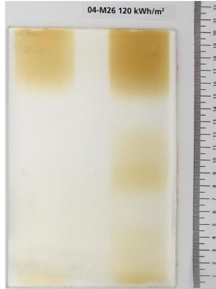
Figure 2: Example of yellowing of a back-sheet below different filters after a UV-irradiation of 120 kWh/m²
