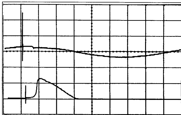
Top trace: Voltage across bulb terminals, 500 V/div Bottom trace: Current in bulb, 50 A/div Sweep: 2 ms/div
