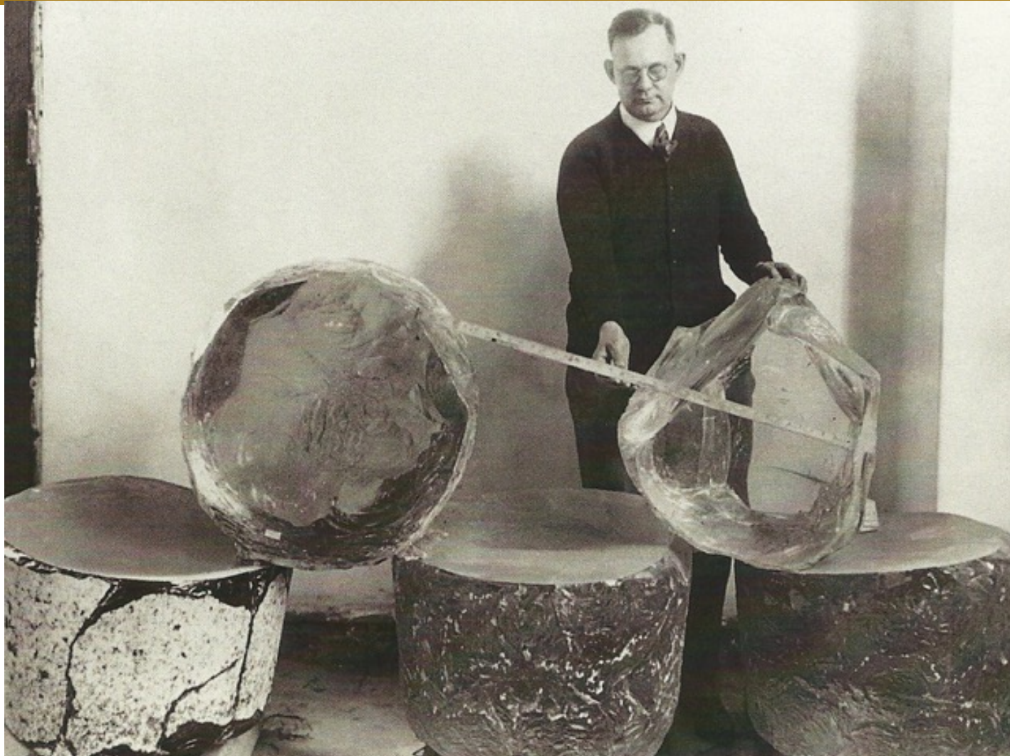
2-foot thick 1000 lb pieces of optical glass created at NBS.
