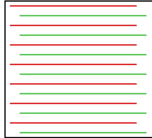
Interlaced – even and odd fields may be offset if subject moves so algorithm must correct
