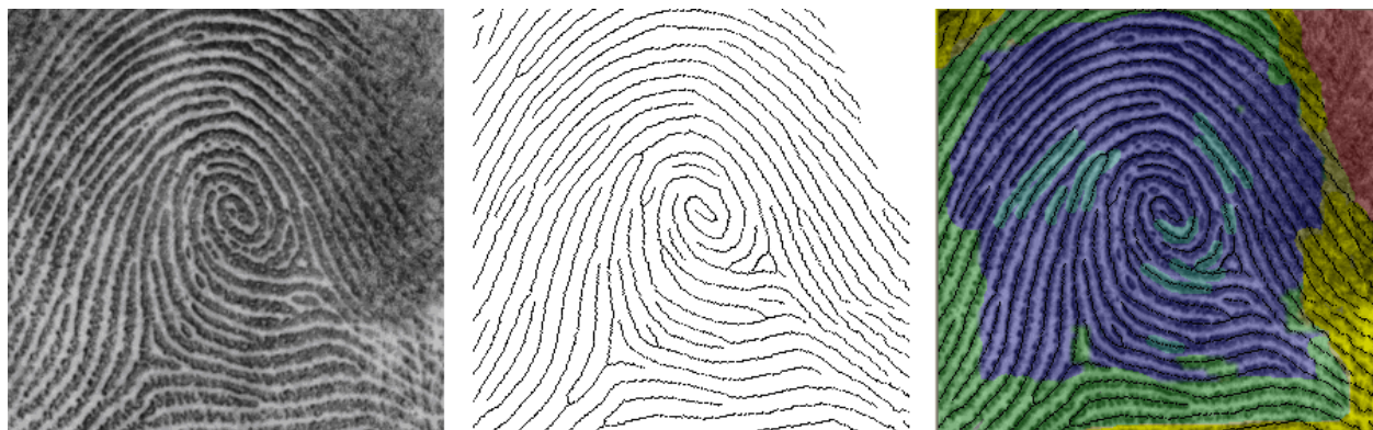
Figure 22: Examples of fingerprint, skeletonized representation, and overlay of original / skeleton / quality map
