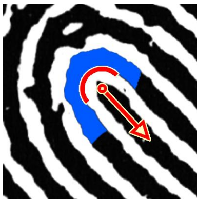
Figure 9: Placement of the core at the focus of the innermost recurving ridgeline
