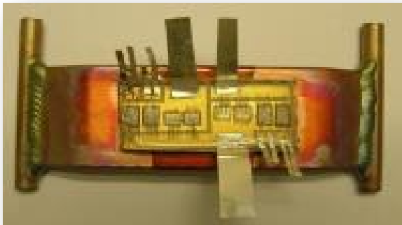
100A/1200V SiC Phase-leg Module with Integrated Cooling
