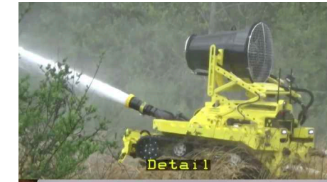
Howe & Howe Thermite RS1 & RS3 550kg (1200lbs) 1200 Gallons per Minute
