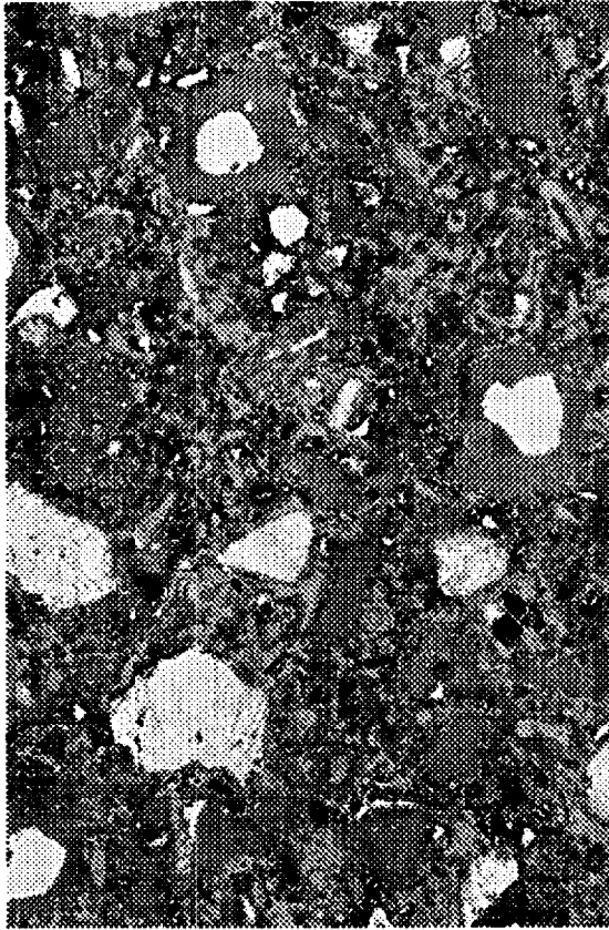
Figure 2: Comparison of real SEM images for saturated (left) and sealed (right) hydration for Cement 115 with w/c=0.3 . Unhydrated cement is white, porosity is black, calcium hydroxide is light grey, and calcium silicate hydrate gel and other hydration products are dark grey. Areas imaged are approximately 128 \mu\text{m} \times 190 \mu\text{m} .
