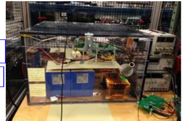
Figure 1 : (a): Leakage current with blocking voltage; (b): Experimental setup of two series connected 15kV SiC IGBT devices; (c) Experimental setup of two series connected 10kV SiC MOSFET devices;
