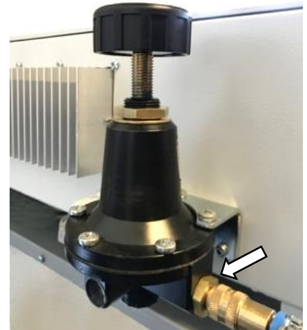
Figure 12: Compressed air connection on the pressure regulator
