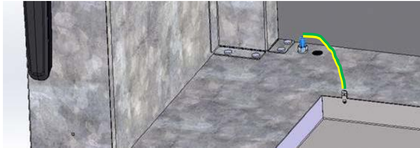
Figure 20: Grounding cable for the equipotential bonding between the condensate collecting tray and the pump module via
