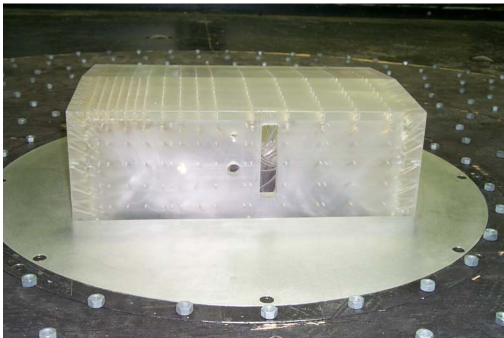
OPENINGS ON THE 40' BUILDING MODEL
