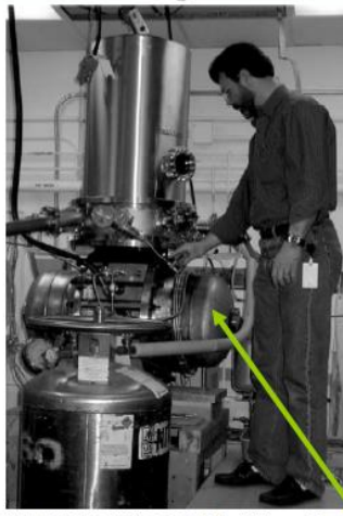
NIST 500 W@30K Stirling-PT cooler
