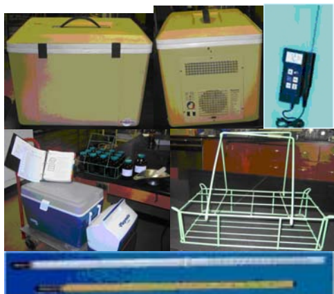
From Top Right – Portable refrigerators; Digital thermometer; Coolers, Documentation and Grain transfer standards; Rack; and Liquid-in-glass thermometers.
