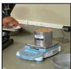
Figure 4. Weighing the quart kettle and grain.
