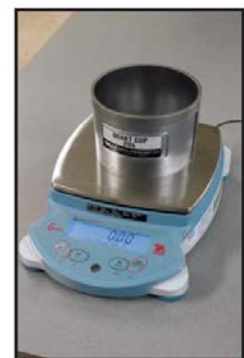
Figure 2. Zero weight of the empty quart kettle.
