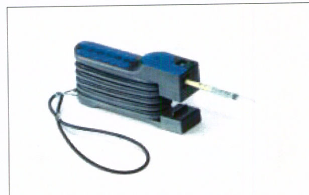
Sorbent tube samplers for workplace gases and vapors are used in a number of standards developed by Subcommittee D22.04.
