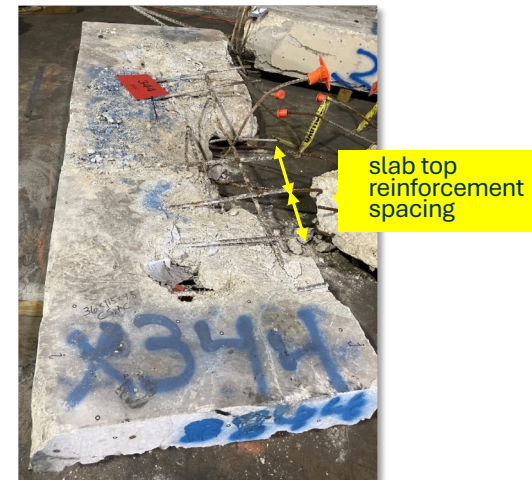
Top Reinforcement in Pool Deck Lower than Design Requirements Placement of Top Bars in Column Strips
