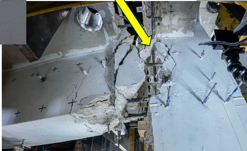
Test #1, column bars at north face lose cover and buckle
