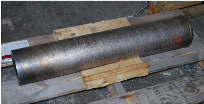
Figure 8.11: As cast 300-lb VIM/VAR heat of QT-Co
