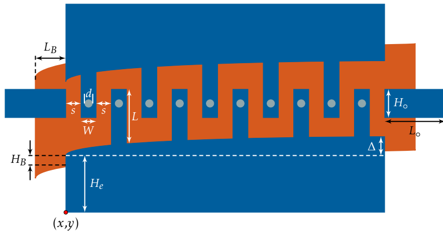
Figure 2.343: Two interacting rectangular arrays between elements of differing lengths. Beam lengths vary non-linearly across the electrode base. Structures are generated using the MARACURVES and MARACURVE constructors.
