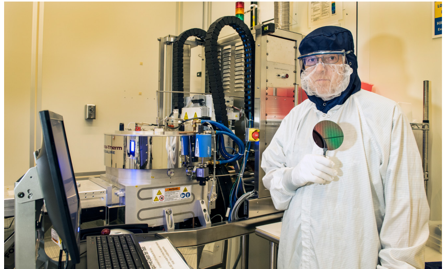
Process Engineer Richard Kasica of NIST's Center for Nanoscale Science and Technology holds a wafer of the type typically used in the plasma-enhanced chemical vapor deposition chamber at center. Credit: NIST
