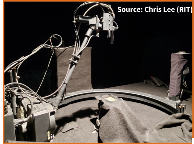
Goniometer of the Rochester Institute of Technology-Two (GRIT-T). Image Credit: C. Lee J. Harms, C. Bachmann, B. L. Ambeau, J. Faulring, A. Ruiz Torres, G. Badura, E. Myers, 2017. "A fully-automated laboratory and field-portable goniometer used for performing accurate and precise multi-angular reflectance measurements," Journal of Applied Remote Sensing , 11(4): 046014-1-046014-15, https://dx.doi.org/10.1117/1.JRS.11.046014 .
