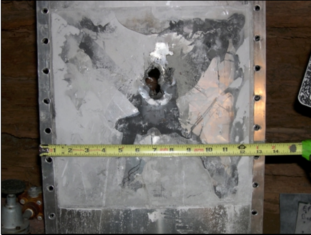
Figure 5-19. Post-Test Damage Image of EPP-06 Enhanced Powder Panel
