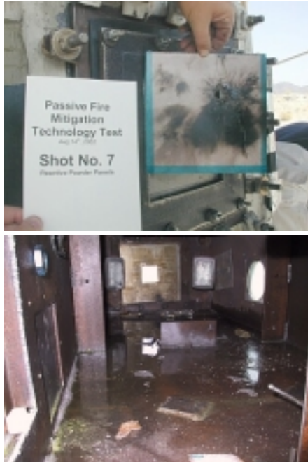
Figure 5-7. Comparison Of Commercial And Enhanced Powder Panel Agent Release In JTCG/AS Dry Bay Fire Extinguishing Testing
