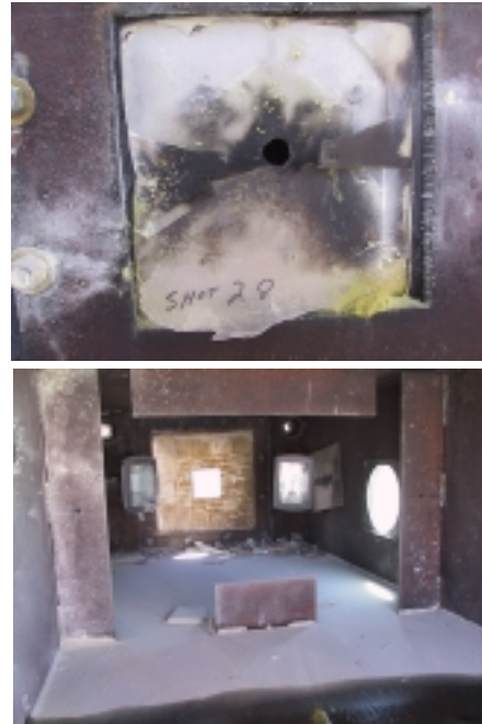
Figure 5-7. Comparison Of Commercial And Enhanced Powder Panel Agent Release In JTCG/AS Dry Bay Fire Extinguishing Testing
