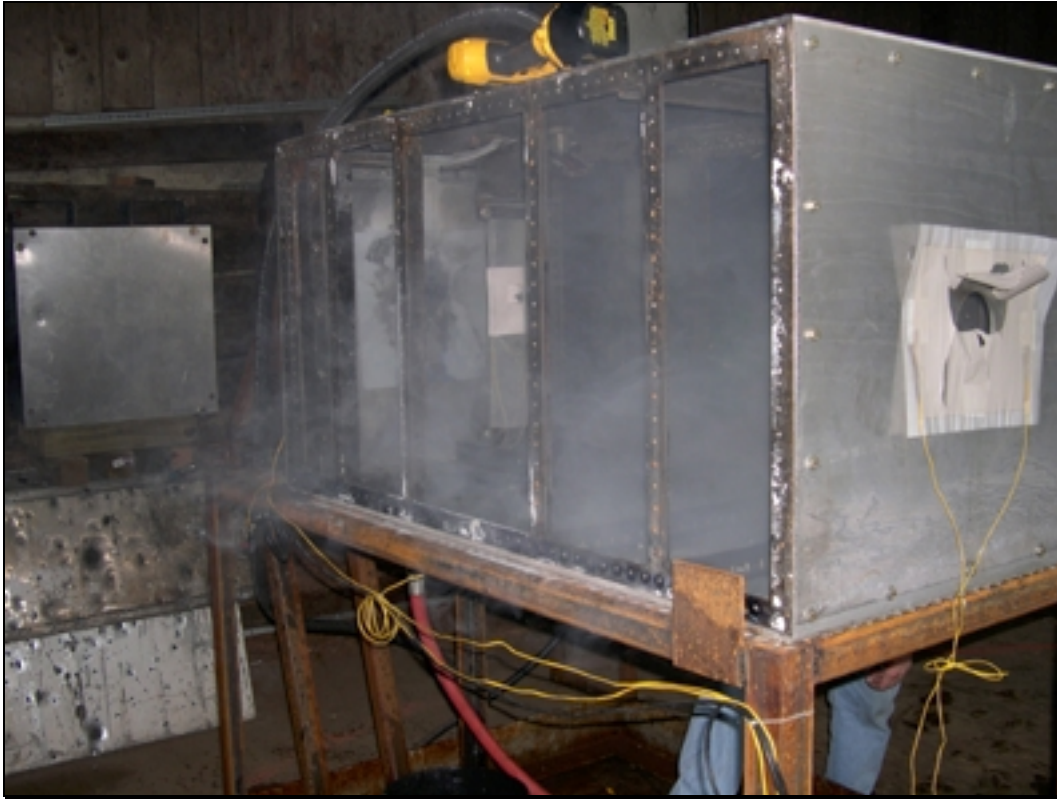
Figure 5-22. Powder Evident in Dry Bay More Than Five Minutes After EPP-09 Test (Side Wall Removed)
