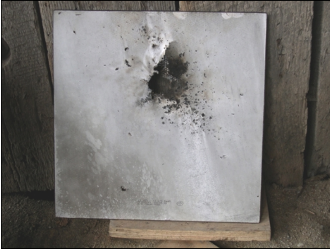
Figure 5-14. Post-Test Damage Image of EPP-03 Commercial Powder Panel
