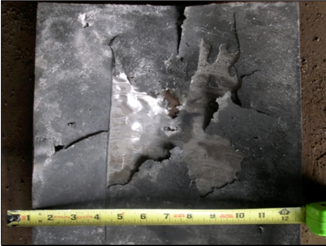
Figure 5-16. Post-Test Damage Image of EPP-05 Enhanced Powder Panel
