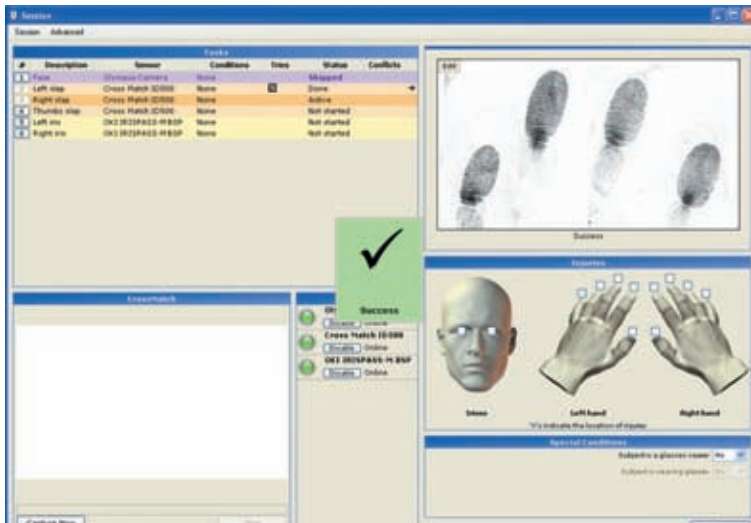
Successful capture. This screenshot shows a successful left slap. The large indicator of success fades away over a few seconds.
