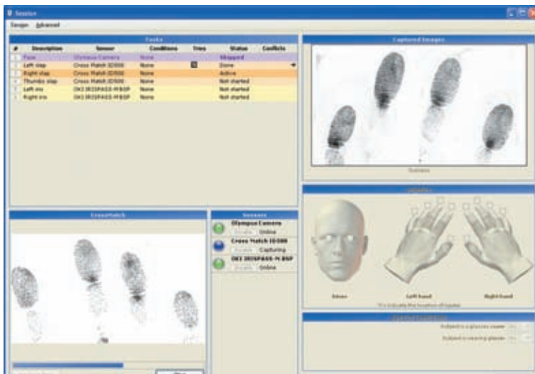
Polling for fingerprints with a live preview. This screenshot shows a right slap in progress. The result from the previous task, a left slap, is visible in the upper-right panel of the window.
