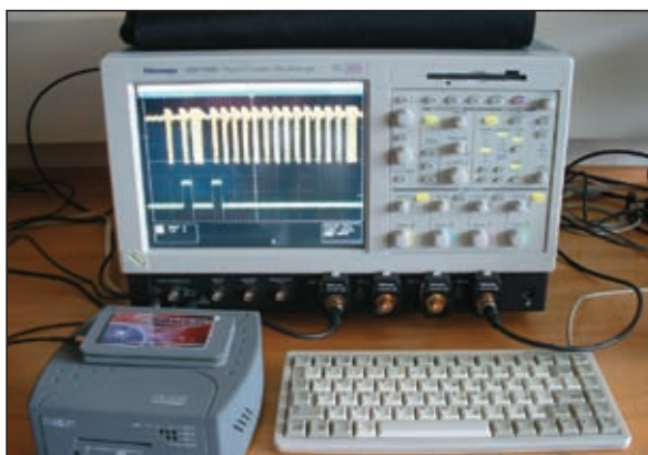
FIGURE 3. Noninvasive Counterfeit Detection Using Waveform Measurements
