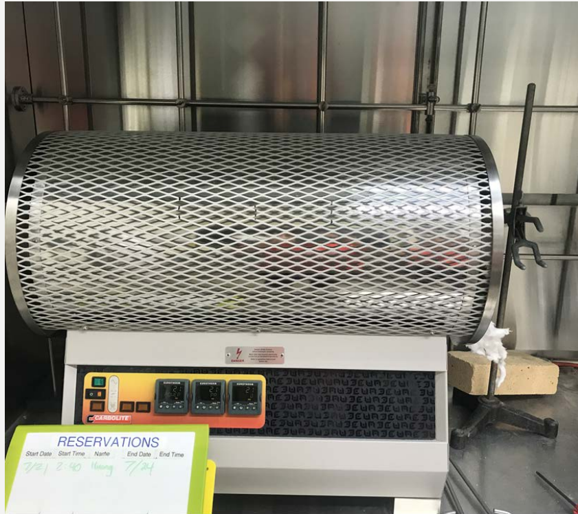
3 zone tube furnace
