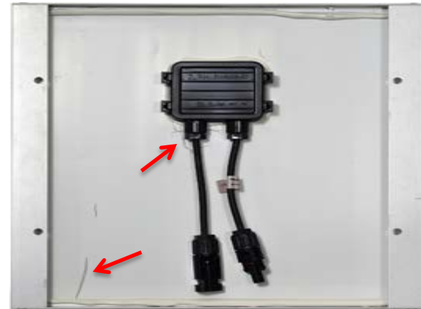
Large cracks in PVDF/PET/FEVE backsheet
