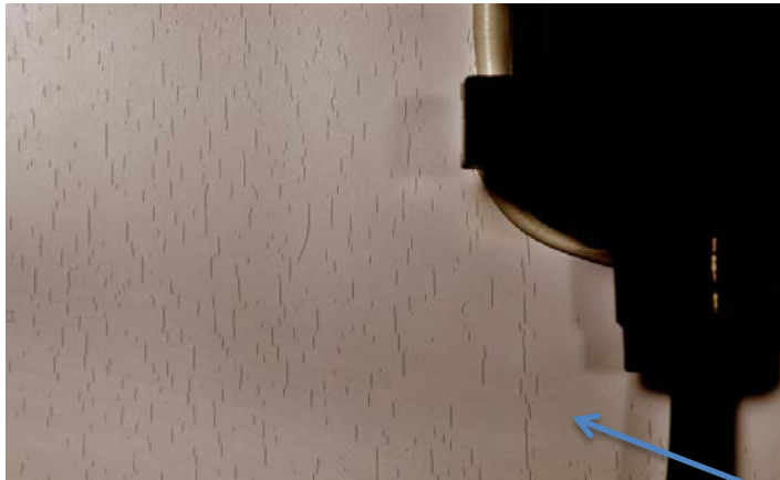
Fine cracking of PVDF layer in PVDF/PET/FEVE backsheet
