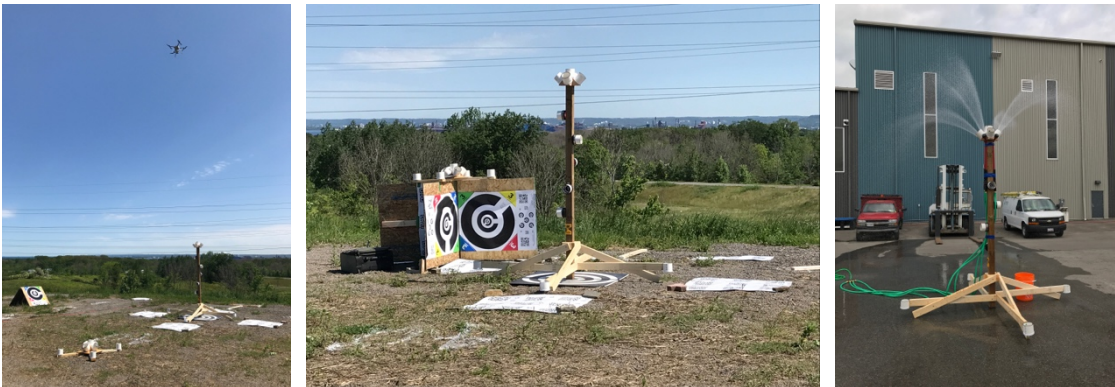
Figure 11: A) The outdoor testing took place in a more remote section of Ontario where the local responders are cleared to fly their systems outdoors. B) We set up our Situational Awareness test methods to practice and validate them using an aerial system manufactured in Canada and used by all the responders. C) Because aerial systems need to handle weather conditions, we adapted a sprinkler system to the Spiral Inspect test apparatus to enable testing resilience of the system to rain.
