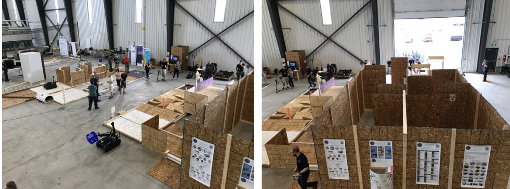
Figure 2: A) The apparatuses set up to the left are the Basic Maneuvering and Dexterity suite of test methods. They are performed sequentially in time limited trials. B) The Access Buildings suite of test methods includes Terrains, Stoops, Stairs, Doors, and Hallway Labyrinths all with embedded Dexterity and Mapping tasks.
