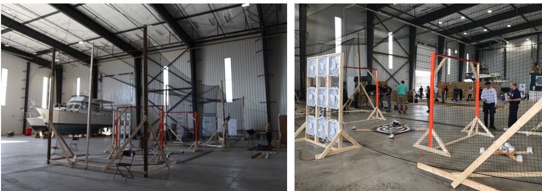
Figure 8: A) The indoor netted aviaries provided safe flight testing while validating the test methods and collecting essential data for the standardization process. B) A wall of fans provided turbulence for the aerial systems, encouraging automatic holding of position and orientation to improve performance of tasks.
