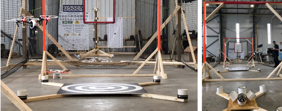
Figure 9: One aviary focused on Maneuvering test methods.
