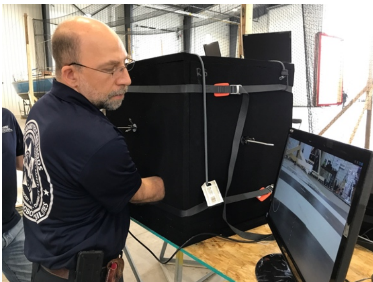
Figure 12: Kam is shown operating an aerial system in the netted aviary from an operator control unit within the new Radio Attenuation test method apparatus. It is essentially a glove box coated with radio attenuation tiles. The signal from the robot is shown on a remote display outside the box. The next revision will contain a camera inside the box so the operator can see his/her own hands as well.
