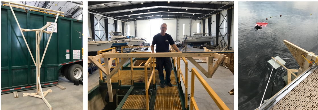
Figure 6: A) The C-frame apparatuses provide five different orientations for each task (0°-45°-90°-135°-180°). B) The walkways on top of the tank appear helpful, but they actually hindered inserting the large apparatus frames into the tank. So open top tanks are preferred. C) The same test methods were replicated off the dock in the brackish water with natural currents and sediment in the harbor. We embed the apparatuses into these operationally relevant scenarios to measure the degradation in performance due to the uncontrolled environmental variables.
