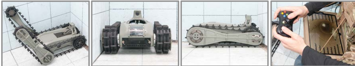
FIGURE 9) Robot configuration identification involves taking pictures of the robot in front of the metered backdrop with 20 cm (8 in) squares. Detail images should capture the sensors, radio, payload locations, operator control unit, etc.
