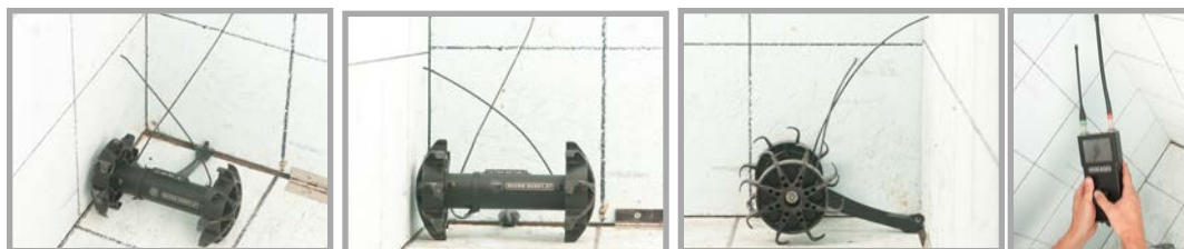
Figure 35) Recon Scout XT, Recon Robotics, Inc., USA (0.5kg / 1.1lbs)
