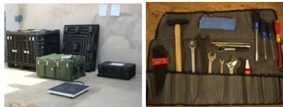
FIGURE 10: A) The robot packaging container sizes and weights should also be documented along with the tool set. Some responders have clear guidelines for how long they should be operational in the field without re-supply. So the number of batteries to pack, for example, is a big issue.
