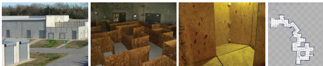
FIGURE 30: Search and map an intact building containing random maze test apparatus within some rooms. Locate any signs of life (visible shape or motion, audible, thermal) and any suspicious packages, hazardous materials, placards, or labels. All objects of interest should be located on a 2-D map of the area with recognizable navigation features.
