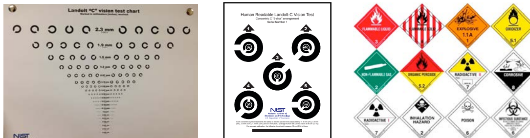
Figure 11: Visual targets are used within the test apparatuses to evaluate the visual and color acuity of robots under test in lighted and dark conditions. A) Landolt C chart for near field vision (far field chart looks similar, but larger). B) Concentric Landolt C charts for embedding into test apparatuses and operational scenarios are generated by NIST so can be scaled to any size. They appear in the 5-dice pattern to emphasize at least some statistical significance. C) Hazardous materials labels, which are 10 cm (4 in) on a side.
