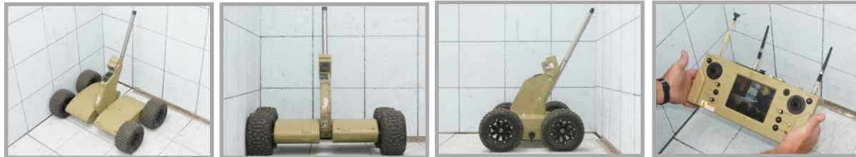
Figure 43) Pointman LRV, Applied Research Associates, Inc., USA (7.9kg / 17.4lbs)
