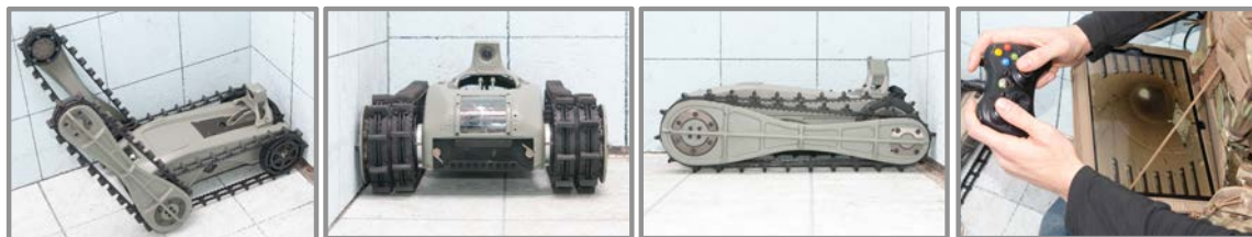
Figure 42) Micro Tactical Ground Robot (MTGR), Roboteam Ltd., Israel (6.5kg / 14.3lbs)
