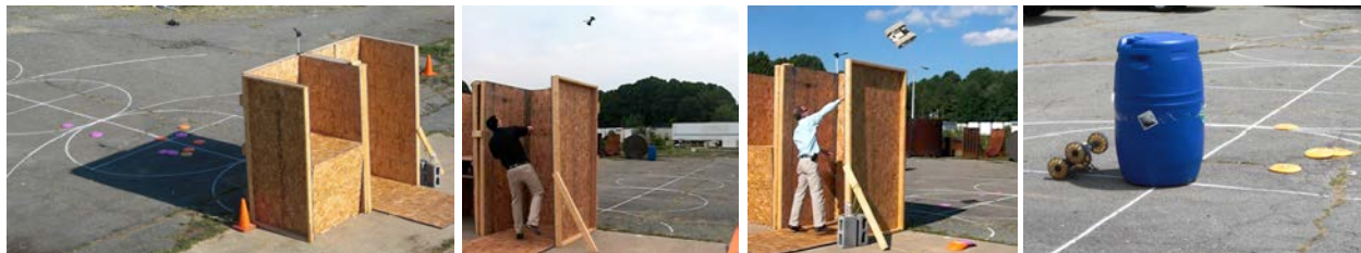
FIGURE 6: A) The draft standard test apparatus Throw Distance includes a 2.4m (8ft) tall wall to throw over, an adjoining remote control station to limit sight lines down-range, and landing locations with 4m (13ft) diameter circular lines for the robot to follow. B and C) Robots may be thrown over the wall in any manner with a two-step approach while staying on the 2.4m (8ft) OSB panel on the ground. D) Hazmat targets are placed at the center of the circle for the robot to identify to demonstrate functionality after each throw. Colored discs on the ground mark the landing locations for each trial which can add up to 30 repetitions.
