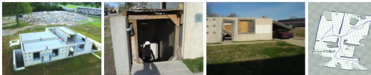
FIGURE 31: Search and map a dwelling with a basement. Locate any signs of life (visible shape or motion, audible, thermal) and any suspicious packages, hazardous materials, placards, or labels. All objects of interest should be located on a 2-D map of the area with recognizable navigation features.
