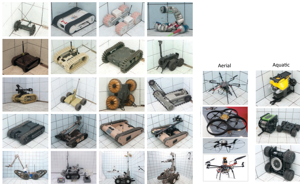
FIGURE 5: Over 100 robots have been tested to varying degrees of completeness across the roster of standard test methods. These are some examples of response robots that show the range of sizes of ground robots, some examples of vertical take-off and landing sUAS, and some small aquatic ROVs that are indicative of the robots targeted within this project.
