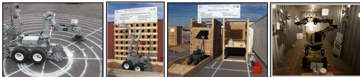
FIGURE 20: A few test methods for larger robots practicing counter vehicle-borne improvised explosive device tasks: A) heavy lifting of objects around the robot, B) tool deployment for cutting access, C) inspecting a vehicle cab and cargo bay, and the D) Pan-Tilt-Zoom Tasks.
