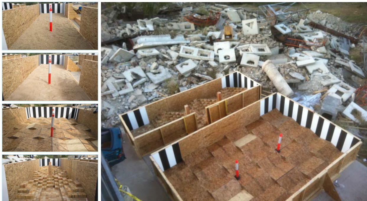
FIGURE 19: Examples of using standard test methods as incrementally complex challenges on the way to more operationally difficult environments like the rubble pile at Disaster City. A robot should be able to complete all the standard terrains to statistical significance prior to trying the rubble. There are lessons to learn in negotiating the Stepfield terrain (shown in the middle distance above), like how to right the robot when it rolls over!
