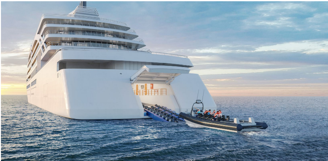
This rendering shows what the new Viking expedition ships will look like, including the hangar for launching small vessels. Credit: Viking
