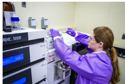
NIST research chemist Kelly Telu injects a sample into a mass spectrometer, a laboratory instrument that scientists use to identify unknown chemical compounds.
