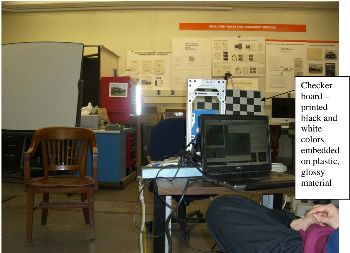
Figure 4. Photo of the experimental set-up with the reflector, illuminated from the camera flash, set at the -1m height and showing the computer laptop data capture system. At this location, the roller table is 3.5 m from the reflector.
