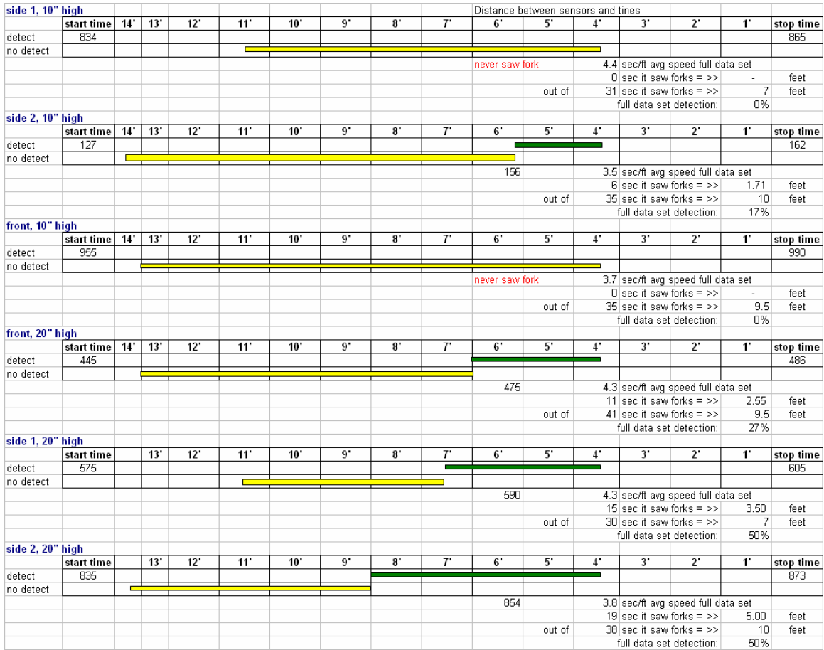
Figure 13: Tine Detect Chart for each of the six data sets graphically showing the detect distances (green bar) of forklift tines and the non-detect distances (yellow bar).
