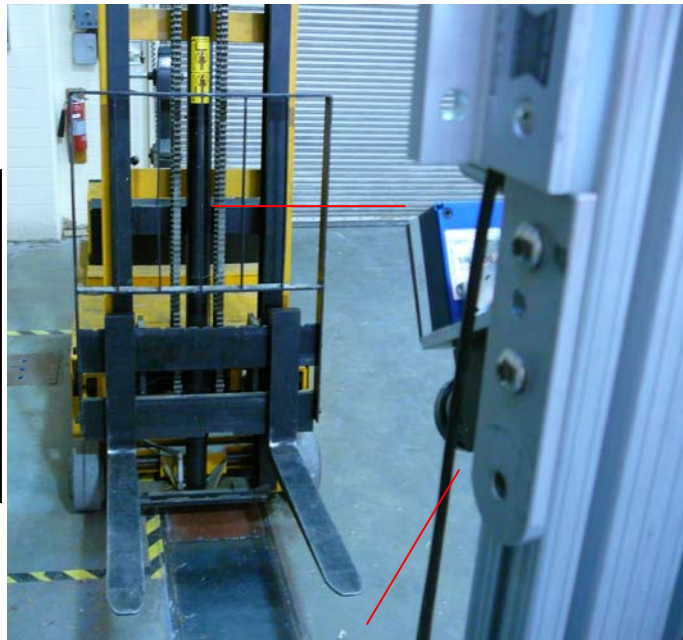
Figure 6a: Camera view of Front Experimental set-up with the SR3000 & Camera viewing the forklift tines. The red lines show an approximate sensor field of view.
