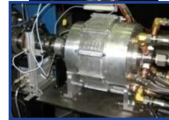
Micro-channel cooling jacket & slot cooling tubes
