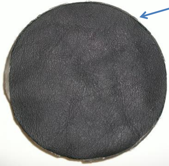
Photo of the top (skin) side of a 10 cm (4") diameter cylindrical shape soft tissue bio-simulant artifact
